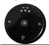
IMPORTANT The barometer must be in the vertical (upright) mounted position. Determine which way you need to adjust the barometer needle (not the pointer). Make a very small adjustment to the rear centre screw with a small screwdriver. Tap the glass firmly, and make another small adjustment. Keep repeating the above procedure until the barometer needle reading matches that obtained from your local source.
